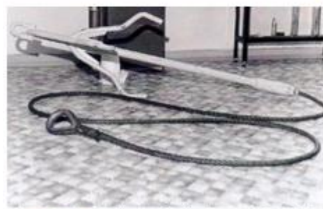
A net cutter, first used in the Second Cod War
